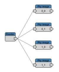
Physical Image element has input and output. The input is used for reader connection. The data goes out of reader to the Physical Image element and saved to dump file. On the output Physical Image connects with other elements for further transformation of physical image to virtual and logical.
