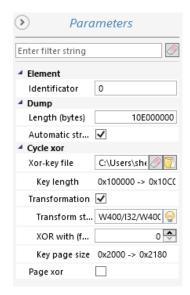
The button 🖻 automatically adjusts the XOR key structure according the page structure (when XOR key for Data area only is used)
