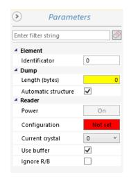
Power ON/OFF turns the power of NAND chip ON/OFF. Pressing the button performs the action displayed on it (not status!). When power is ON, the yellow LED of reader is alight.
