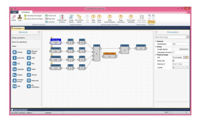
Elements represent the operations for transformation of the physical image of Nand memory chips. Elements are added to the workspace by Drag&Drop method. The set of elements is divided into several types: Dump operations, Block list operations, other elements.
